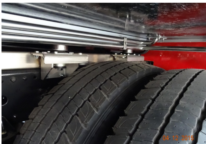
Stainless steel subframe, stainless steel water pipe
